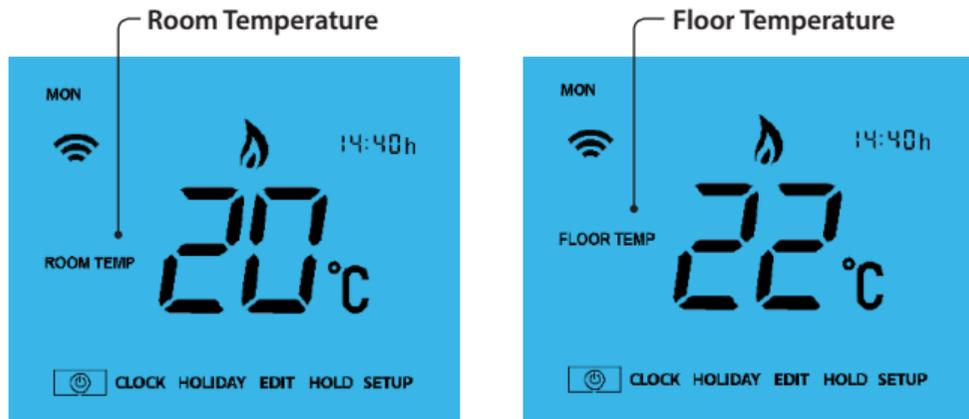
When the ProTouch iQ is set to use both the air & the floor sensor, the room temperature will be displayed by default.
