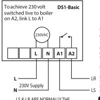
LS & LR ARE NORMALLY THE ROOM THERMOSTAT CONNECTIONS
