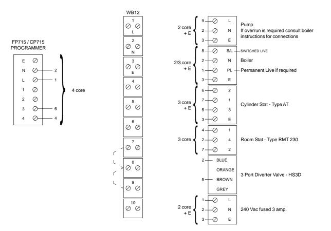
If a room thermostat is not being used then link terminals 4 and 7 on WB12. N.B. Set switch No. 2 on the back of the FP715/CP715 to the 'gravity' position.
